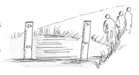
'be alert' and red nearer the top, meaning 'danger'. This gives an indication of how quickly the water is rising. During heavy rain, some community members should be given the task of monitoring the water level and warning the community if the water reaches the danger level (marked in red).
