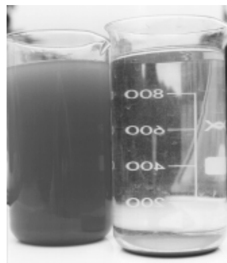
Untreated river water (left) after 2 hours settlement. On the right is water treated with moringa seed solution and left to settle for 30 minutes.
