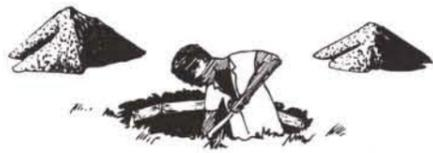
As you dig, throw the soil well away from the hole, so that it doesn't fall back in the pit. First dig a trench for a foundation for your latrine slab. This need only be two or three courses of brick deep (or one concrete block). Build the foundation wall, let it become hard and then dig your pit down inside the foundation wall.
