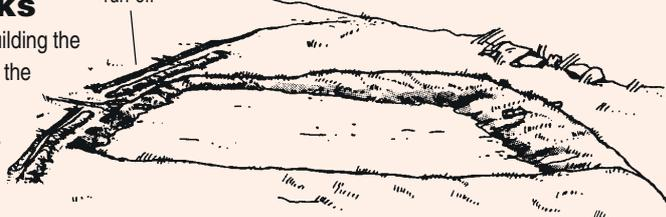
At heavy rains, dig a run off ditch along the upper side of the pond to carry water away from the pond, preventing damage to the walls.
