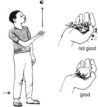
from the bottom. Moisten this soil and squeeze a handful of it into a ball, throw it about 50cm into the air and then catch it. If the ball falls apart in your hand this means it is not good for building ponds. Look for another site or use one of the methods of lining ponds described on page 5. If the ball holds together it probably has enough clay for a fish pond.
