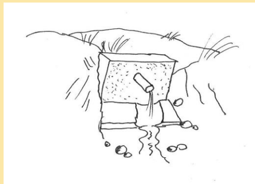
Spring (water source) protection
