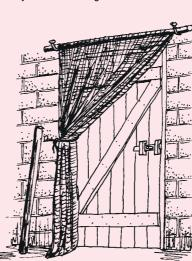
If the house rafters are exposed, mosquitoes can enter easily. • Make lightweight wooden frames and cover with local matting for a cheap but effective ceiling. Check for cracks and fill with scraps of netting. Alternatively, hang treated netting to cover the gap between
