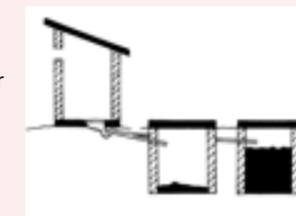
**Ecological sanitation** Ecological sanitation (eco-san) involves using the contents of the latrine for agriculture, after it has been treated to ensure it is not harmful to health. There are various types of eco-san including:
