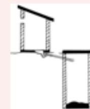
**Pour flush twin pit** This is the same as the pour flush single pit latrine, but there are two offset pits so that once one pit is full, excreta can be diverted to the other pit. After one year the full pit can be emptied and used again while the other is sealed and the contents allowed to decompose. The latrine is therefore permanent.
