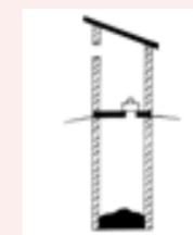
**Single pit ventilated** A single pit is dug. A vertical ventilation pipe is installed which takes away the smell. Wind blowing across the top of the pipe sucks air out of the pit while fresh air flows into the pit through the squat hole, which must be left uncovered. To control flies, the shelter must be kept dark and the ventilation pipe should have mesh fitted over the top.
