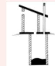
**Twin pit ventilated** Two pits are dug next to each other. The shelter is built partly over both pits. One pit is used at a time. Once a pit is full, it is sealed. The pipe is moved to the other pit and the other squat hole is opened. After one year, the full pit can be safely emptied and the contents used as manure.
