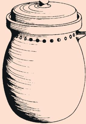
THE SHITAL POT was developed by the Ceramic Unit, Centre of Science for Villages, Wardah, India and can easily be made by a village potter. The inner pot is glazed or waxed to make it watertight. It rests inside the rim of the outer porous pot. The heat of the day causes water to evaporate and escape through the holes below the lid of the pot as well as through the pot itself. This cools the inner storage pot and its contents.
