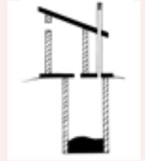
**Twin pit ventilated** Two pits are dug next to each other. The shelter is built partly over both pits. One pit is used at a time. Once a pit is full, it is sealed. The pipe is moved to the other pit and the other squat hole is opened. After one year, the full pit can be safely emptied and the contents used as manure.
