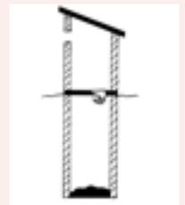
**Pour flush single pit offset** A single pit is dug and the shelter is built a small distance away ('offset'). A waterseal pan and pipe is installed. More water is needed to flush because the excreta has further to travel to the pit, but the advantage of an offset pit over a direct pit is that the latrine can be located in a house and the pit is outside so that it is accessible for emptying.
