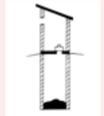
**Single pit ventilated** A single pit is dug. A vertical ventilation pipe is installed which takes away the smell. Wind blowing across the top of the pipe sucks air out of the pit while fresh air flows into the pit through the squat hole, which must be left uncovered. To control flies, the shelter must be kept dark and the ventilation pipe should have mesh fitted over the top.
