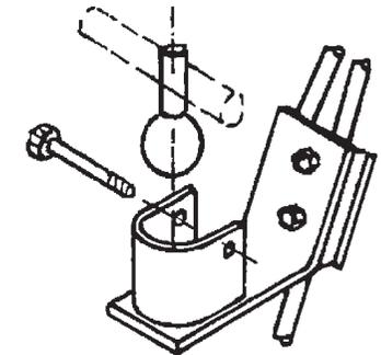
Hitch design. A steel or rubber ball drops into a socket formed from a flat bar or cut from a pipe bolted to the carrier or frame of the bicycle.
